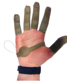
Figure 1. Instrumented glove (Finger Tips Sensor-PPS).
